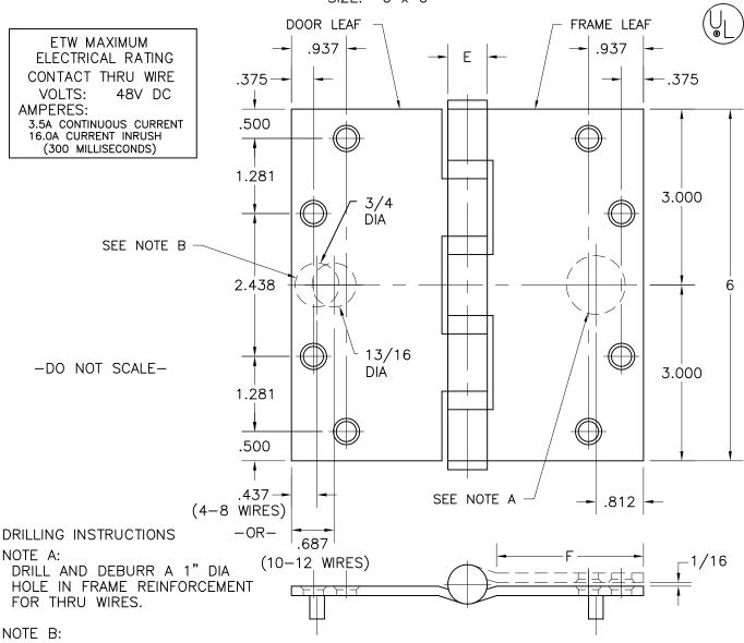
DRILL AND DEBURR A 3/4" DIA HOLE FOR 4-8 THRU WIRES -OR-A 13/16" DIA HOLE FOR 10-12 THRU WIRES IN DOOR REINFORCEMENT.
