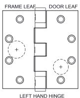
HINGES ARE NON-LOAD BEARING AND MUST BE MOUNTED IN THE CENTER POSITION ONLY.
