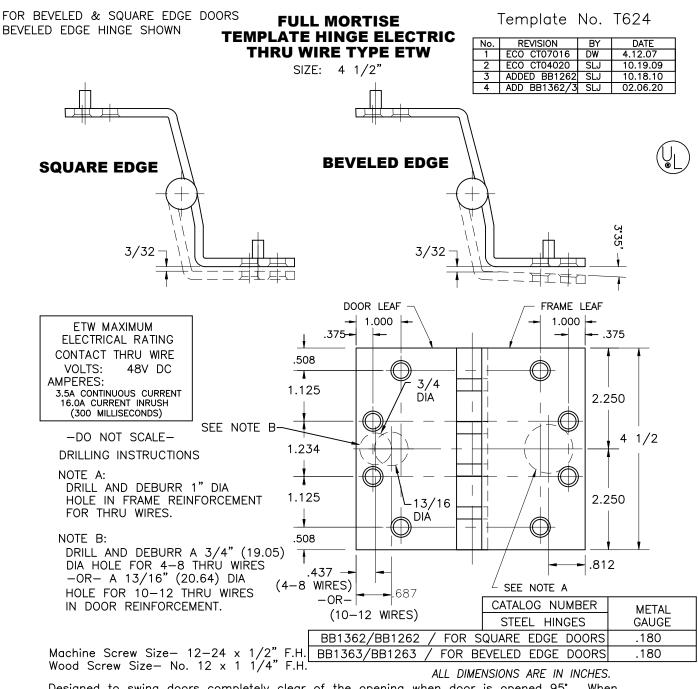
Designed to swing doors completely clear of the opening when door is opened 95°. When opened 90°, door projects 11/64 (4.37) past stop of jamb.
