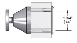
NOTE: STANDARD SINGLE GANG BOX WILL NOT WORK WITH 380R WITHOUT MODIFICATIONS. USE HAGER 381B GANG BOX TO INSURE PROPER INSTALLATION.
