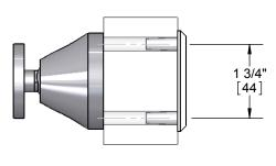
NOTE: STANDARD SINGLE GANG BOX WILL NOT WORK WITH 380F WITHOUT MODIFICATIONS. USE HAGER 381B GANG BOX TO INSURE PROPER INSTALLATION.
