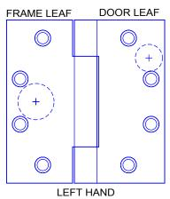
HINGES ARE NON-LOAD BEARING AND MUST BE MOUNTED IN THE CENTER POSITION ONLY.
