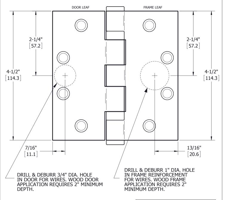
HINGES ARE NON-LOAD BEARING AND MUST BE MOUNTED IN THE CENTER POSITION ONLY.
