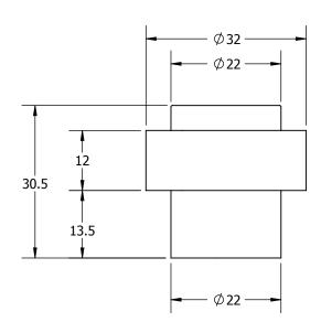
FASTENERS: 1PC #5 X 30mm WOOD SCREW 1PC NYLON FINNED PLUG ANCHOR
