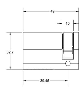
NOTE: DRILLED SEVEN PIN HAGER 'H1' KEYWAY
