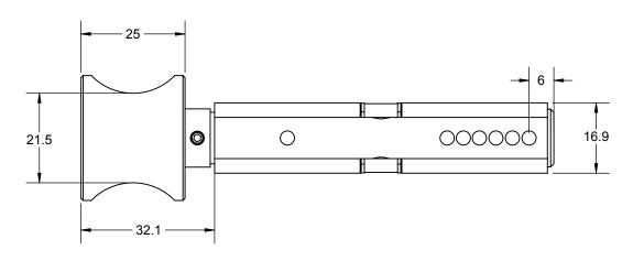
NOTE: DRILLED SIX PIN SCHLAGE 'C' KEYWAY
