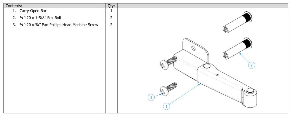
The **297C Carry-Open Bar** pushes the active door beyond the door coordinator's hold-open position. The 297C Carry-Open Bar is not needed when the inactive door is equipped with flush bolts.
