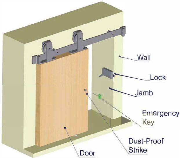
Installation based on barn door application where doors are hung on the **OUTSIDE** of the room.
