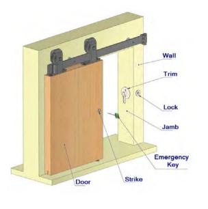
Installation based on barn door application where doors are hung on the **OUTSIDE** of the room.
