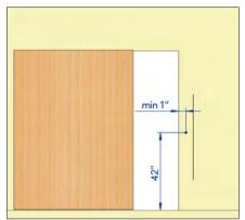
For drywall opening with 1/2" drywall (gypsum board), minimum 2" door overlap is needed to install BD4000 privacy lock. The lock bore center must be at least 1" from wall edge; align strike with lock.
