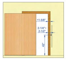
Do not install lock on casing that is less than 1-5/8" wide. Drill lock bore at least 2-1/4" from edge. For this type of installation, door overlap must be at least 3". Align strike with lock.
