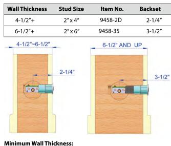
9458-2D - minimum thickness: 9458-2D - minimum thickness 4-1/2" 9458-35 - minimum thickness 6-1/2" There is no maximum thickness for either lock.
