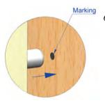
6.1) Move the Barn Door to the Closed position; throw the lock bolt to mark the exact strike center position. Make sure this location is minimum 1" to the edge of the door.
