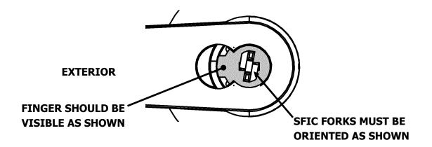
STEP 3: Install SFIC Core in lever
