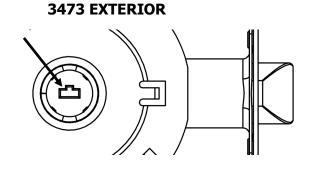
**STEP 2:** Orient the tailpieces in the mating spring cages to match the cams above. Install the exterior spring cage first, followed by the interior spring cage, lining up the cams and tailpieces so they mate together. Do not force the fit.
