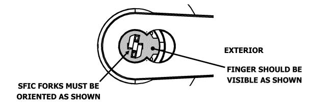
STEP 3: Install SFIC Core in lever
