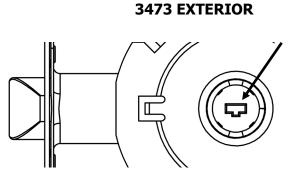
**STEP 2:** Orient the tailpieces in the mating spring cages to match the cams above. Install the exterior spring cage first, followed by the interior spring cage, lining up the cams and tailpieces so they mate together. Do not force the fit.
