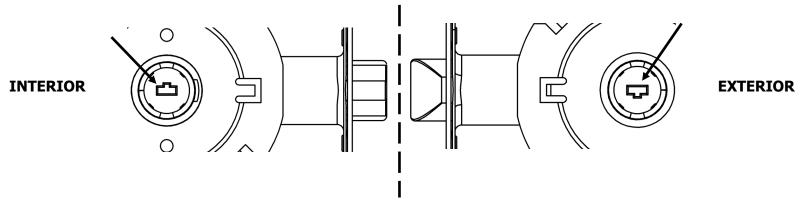
**STEP 2:** Orient the tailpieces in the mating spring cages to match the cams above. Install the exterior spring cage first, followed by the interior spring cage, lining up the cams and tailpieces so they mate together. Do not force the fit.
