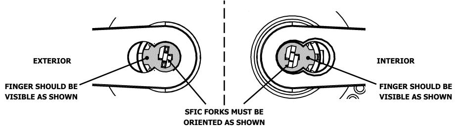
**STEP 3:** Install SFIC Cores in both levers
