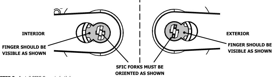
**STEP 3:** Install SFIC Cores in both levers
