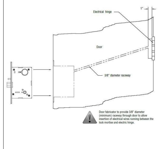
Follow mortise exit device lock body instructions and template to prepare door and frame for installation. Since the motor is located inside the lock body, there are no special preparations or alterations to the standard installation except for the raceway to route wires.
