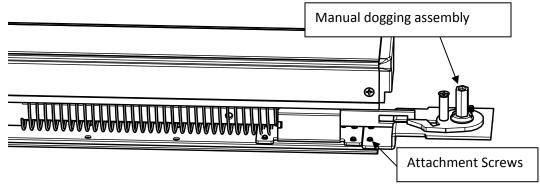
4. Attach the mounting plate of (2-649-5007) MLR kit to the Mechanism Housing Assembly Baseplate using the supplied screws through the holes that secured the manual dogging assembly.
