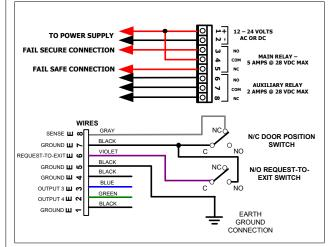
Fig. 4 Basic Door Installation Wiring
