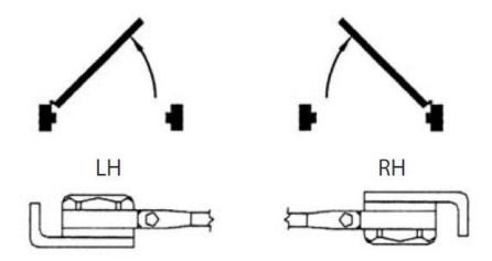
Adjust by loosening hold-open nut, then open door to desired position and tighten hold-open nut securely.
