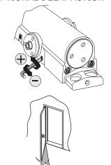
Adjust delay action accordingly to obtain desired delay time.
