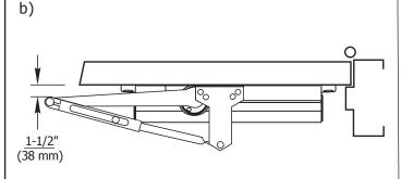
Rotate main arm until the pivot point is 1-1/2" from door surface.
