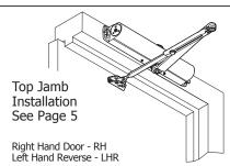
• These door closers should **NOT** be installed on the exposed side (weather side) of exterior doors.
