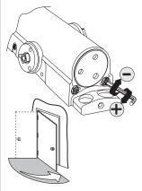
**Note:** Adjust closing time speed to between 3 and 7 seconds from 90° to 0°. Greater closing times may be required for elderly or handicapped.
