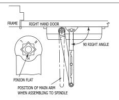
Slide connecting rod into forearm of main arm. Tighten down forearm screw.
