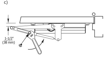
While holding arm in this position, tighten down forearm screw.
