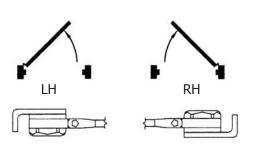
Adjust by loosening hold-open nut, then open door to desired position and tighten hold-open nut securely.
