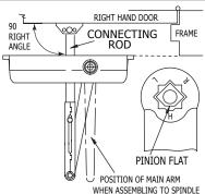
Slide connecting rod into forearm of main arm. Rotate main arm until connecting rod is at a 90° angle to frame. While holding arm in this position, tighten down forearm screw.
