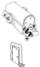
Adjust latch speed so door completely closes and latches.
