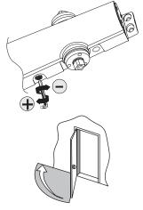
Adjust backcheck accordingly to prevent excessive opening speed.
