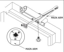
Orient main arm so that the "H", located on the main arm, lines up with the flat on the spindle. Press arm down on spindle and secure with spindle bolt.
