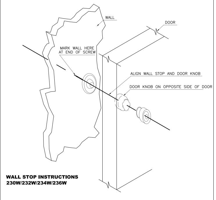
TOOLS REQUIRED: 5/16" DRILL BIT (STD. ANCHOR), 3/8" DRILL BIT (TOGGLE ANCHOR)
