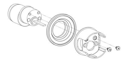
STEP 1: Insert the SALTO GEO cylinder into the Cylinder Collar
