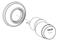
**STEP 2:** Put the Fire Shield onto the back of the GEO Cylinder, lining up the mounting holes
