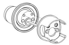
**STEP 3:** Install the two  $\#8-32 \times 1/4$ " mounting screws from the screw pack into the top 2 mounting holes in the cylinder through the fire shield.
