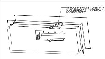
• If using a drop plate, screw the drop plate to the door using 1/4-20 screws. Screw closer to the drop plate using 7/16" long machine screws.
