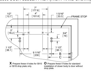
Locate the arm and degree of opening for this installation. Use the chart below to mark/drill/tap (4) 1/4-20 holes for the door. Also, mark/drill/tap (5) 1/4-20 holes in the frame soffit and/or rabbet.
