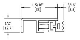
8-32 x 1" PAN HEAD PHILLIPS MACHINE SCREWS (FACTORY PROVIDED) 8-18 x 1" UNDERCUT FLAT HEAD PHILLIPS SHEET METAL SCREWS (FACTORY PROVIDED)
