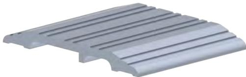
Varying heights are available for most thresholds, depending on the type of extrusion dies used. Different finishes and patterns can also be impressed into the surface to provide extra grip. Other styles beyond the simple saddle threshold are also available. A panic or ADA threshold has a protrusion with a rubber gasket that juts from the surface. This provides a better seal in the doorway.
