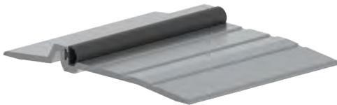
Thresholds are also able to perform more complex functions. A thermal barrier threshold has a PVC spine encased within the middle of the extruded aluminum, connecting two separate pieces. The rubber transmits less heat than a solid aluminum piece and thus keeps the exterior temperature, low or high, from being transferred to the interior of a building.
